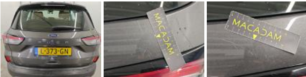
Rear light R tailgate, Scratch(es), Replace
