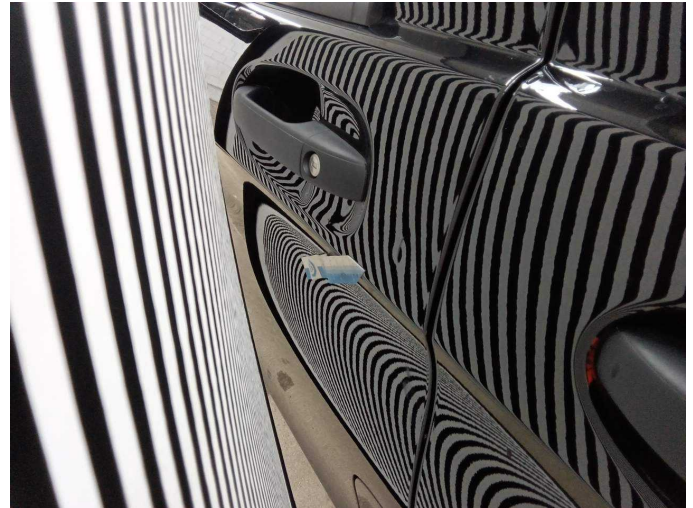
Damage 3: Door - front left side: Door - Dent / paintcoat damage - Smooth repair work
