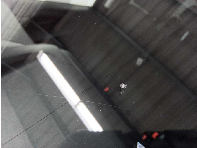
Damage 11: Vehicle glazing: Windscreen (kein Staubschutz) - Stone chips - repair according to calculation
