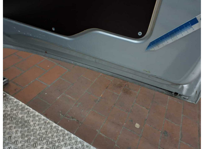
Wear and tear 5: Boot lid / rear door: Rear door - right side (innen) - Scratch(es) - No deduction
