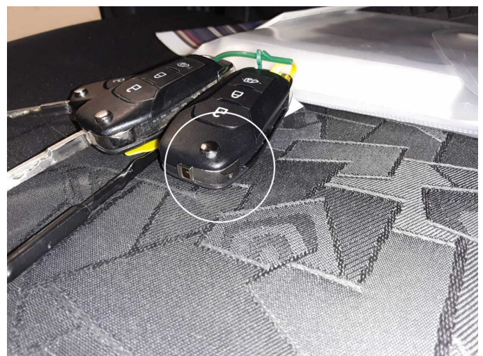
Damage 5: Equipment: Vehicle key with remote control (Schlüssel-bart) - Broken / torn - Replace
