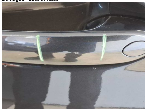
Damage #3: Door - front left side: Door handle - outside - Scratched - Smart repair
