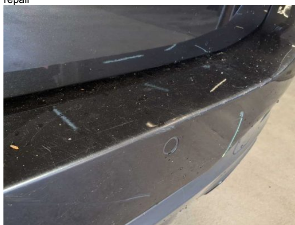
Damage #7: Rear bumper: Rear bumper - Scratched - Smart repair
