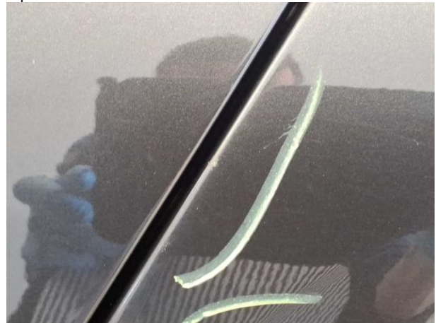
Damage #8: Side panel - rear left side: Side panel - Scratched - Smart repair
