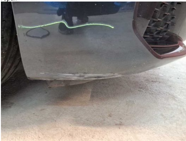
Damage #9: Front bumper: Front bumper - Scratched - Smart repair
