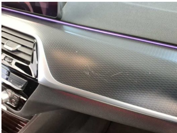
Damage #1: Trim / covers: Brightware / decorative strip - Scratch... - Loss in value
