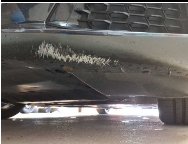
Damage #9: Front bumper: Front bumper - Scratched - Smart repair
