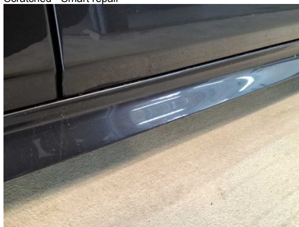
Damage #5: Sill - right side: Trim - Scratched - Loss in value
