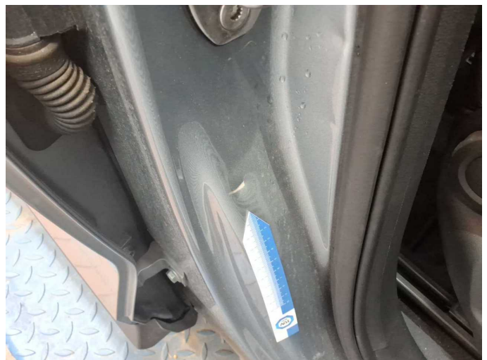
Damage 6: Sill - right side: Sill - dent(s) - Smart repair
