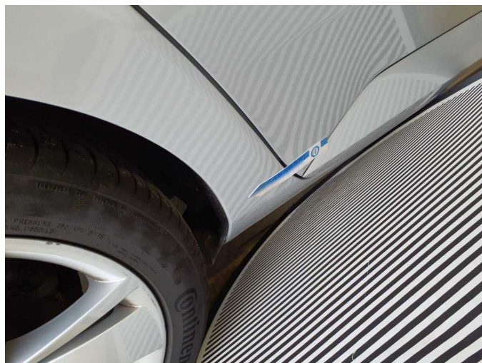
Damage 10: Side panel - rear right side: Side panel (Spachtelmasse eingefallen) - Unprofessionally repaired - Repair and paint
