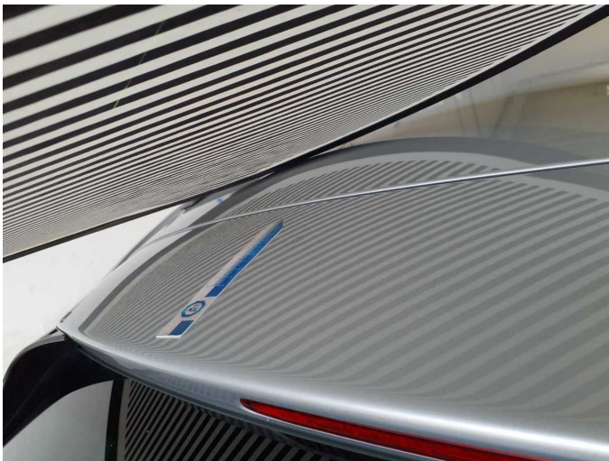
Damage 9: Body: Body - Damage by hail - Repair
