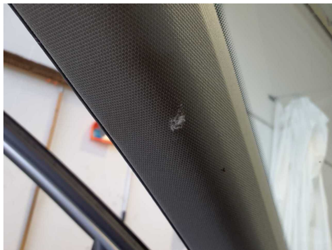
Damage 7: Trim / covers: A-pillar - trim - interior, left side - Scratch(es) - Replace
