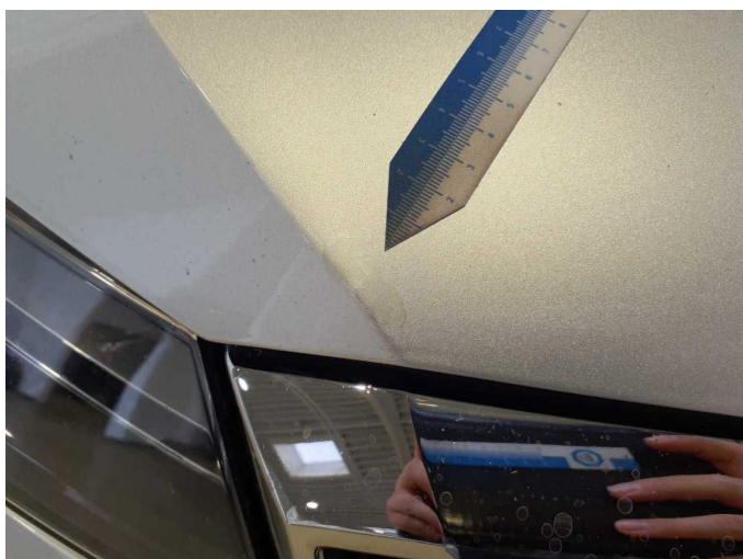
Damage 11: Bonnet: Bonnet (Lackstift) - Paint defect - Paint
