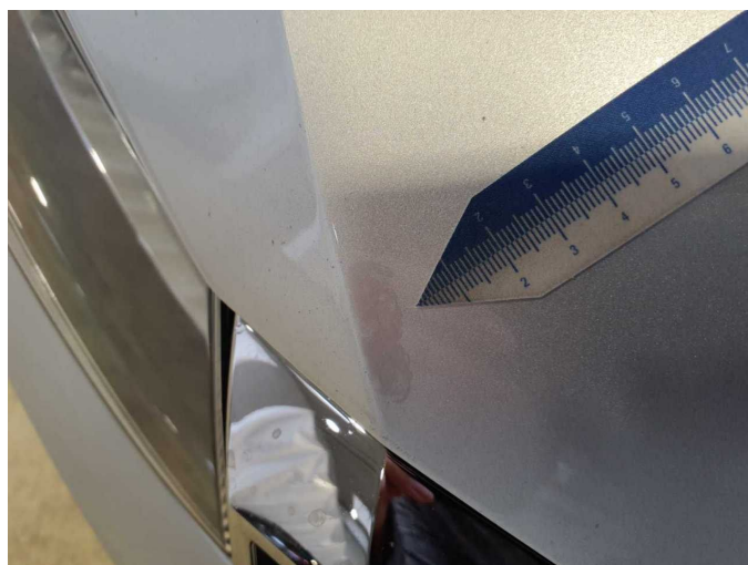
Damage 11: Bonnet: Bonnet (Lackstift) - Paint defect - Paint
