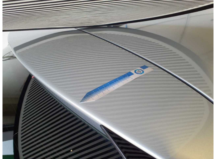
Damage 9: Body: Body - Damage by hail - Repair
