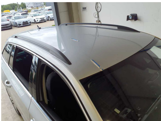
Damage 9: Body: Body - Damage by hail - Repair
