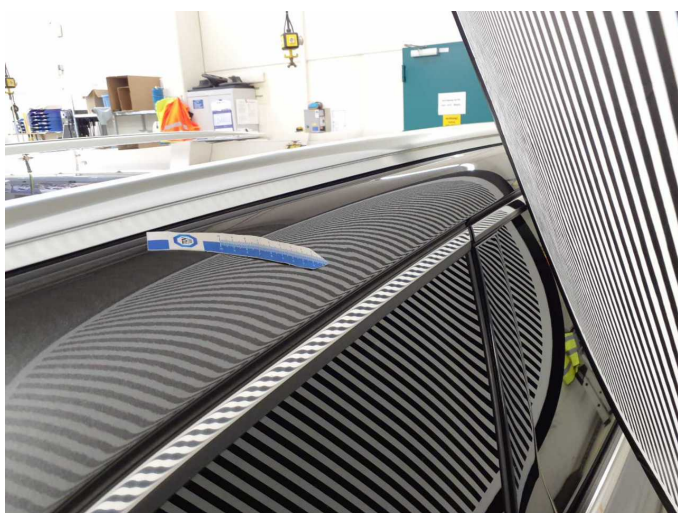
Damage 3: Roof: Roof rail - right side - dent(s) - Smart repair
