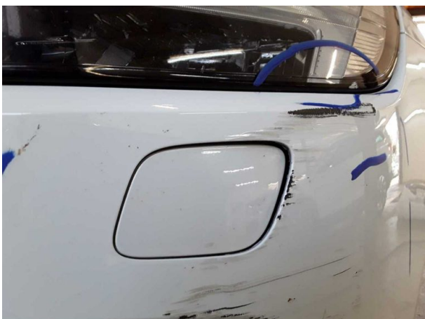
Damage #7: Trim / covers: Trim / covers - Loose - Replace
