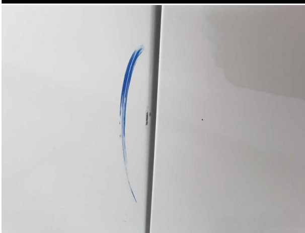
Damage #8: Door - rear right side: Door - Dent / paintcoat damage - Smart repair
