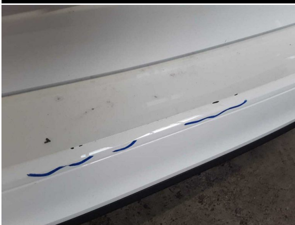
Damage #10: Rear bumper: Rear bumper - Scratched - Smart repair
