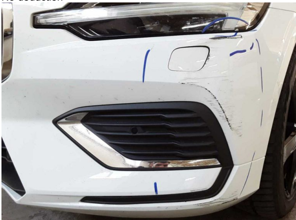
Damage #6: Trim / covers: Trim / covers - Scratched - Replace
