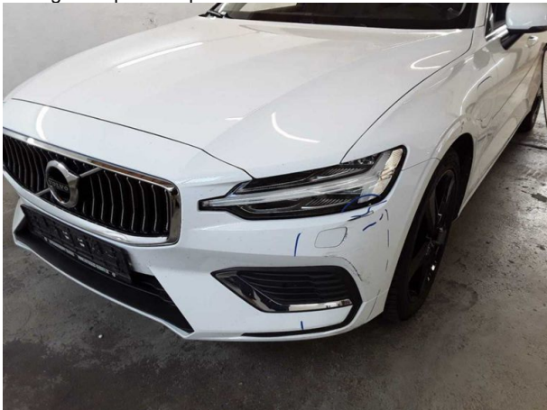
Damage #13: Headlight: LED headlight left - Scratched - Replace
