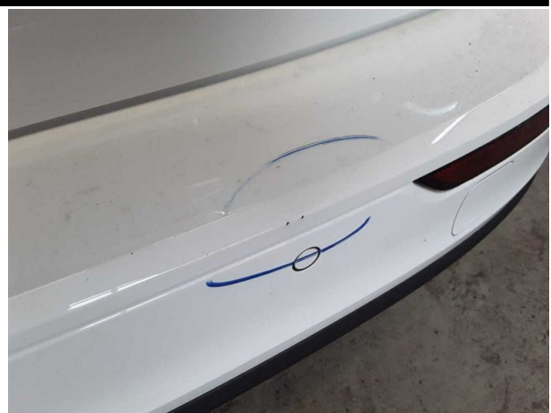
Damage #10: Rear bumper: Rear bumper - Scratched - Smart repair
