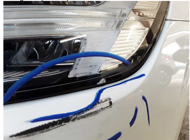
Damage #13: Headlight: LED headlight left - Scratched - Replace
