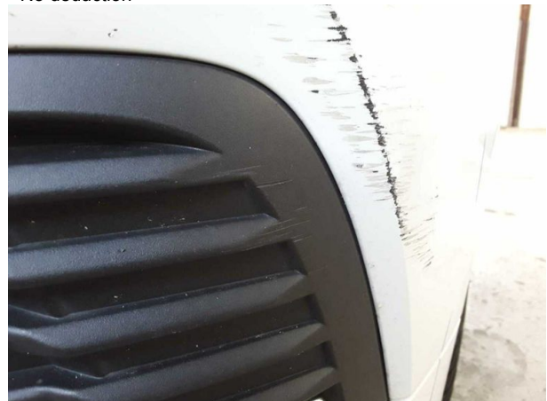
Damage #6: Trim / covers: Trim / covers - Scratched - Replace
