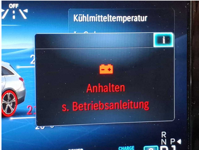
Damage 1: Electrical system: Battery - Empty - Perform diagnosis
