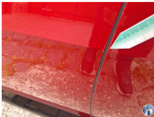
1. Tür Vorne - Links Kratzer - Smart Repair
