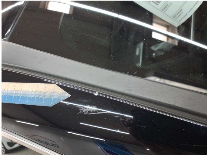
Damage 1: Roof: Roof rail - right side - Stone chips - Smart repair
