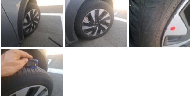
Tyre RR, Out of tolerance, Replace
