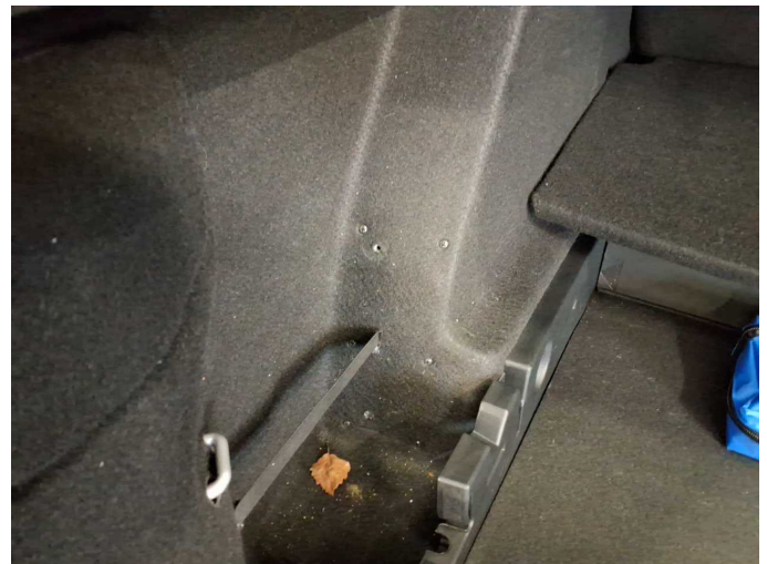
Damage 5: Trim / covers: Cargo area - lining -left side (Fehlbohrungen) - Damaged - Replace
