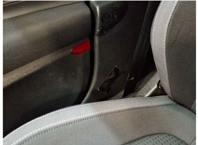
Damage 4: Trim / covers: B-pillar - trim - interior, right side (Fehlbohrungen) - Damaged - Replace
