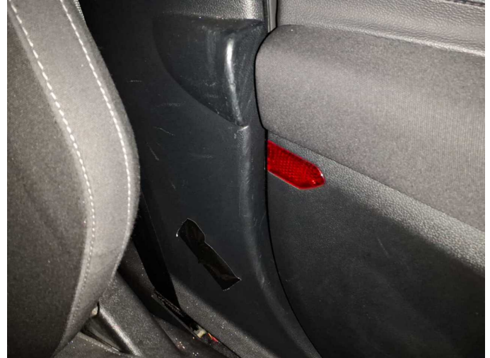
Damage 3: Trim / covers: B-pillar - trim - interior, left side (Fehlbohrungen) - Damaged - Replace
