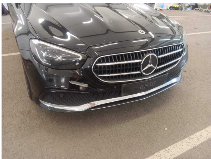
Damage 4: Front bumper: Front bumper - Scratch(es) - Paint
