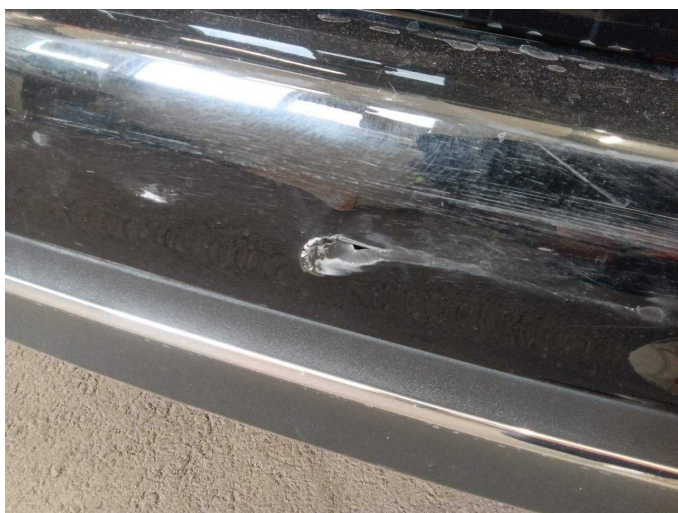
Damage 6: Rear bumper: Rear bumper - Broken / torn - repair according to calculation
