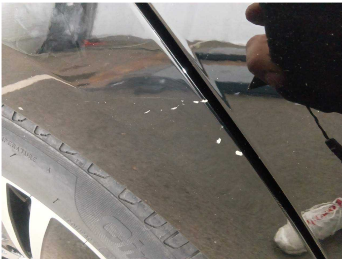
Damage 1: Side panel - rear right side: Mudguard - rear right side - Scratch(es) - Smart repair
