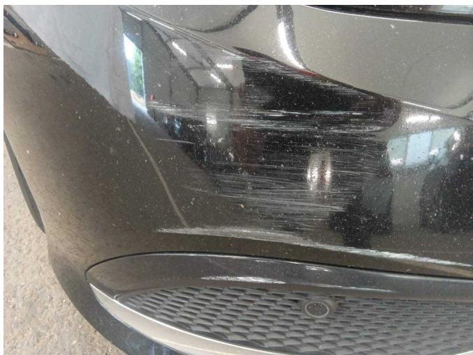
Damage 4: Front bumper: Front bumper - Scratch(es) - Paint
