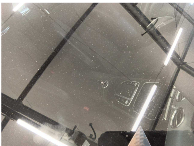
Damage 5: Vehicle glazing: Windscreen (Mit Rissbildung) - Stone chips - repair according to calculation
