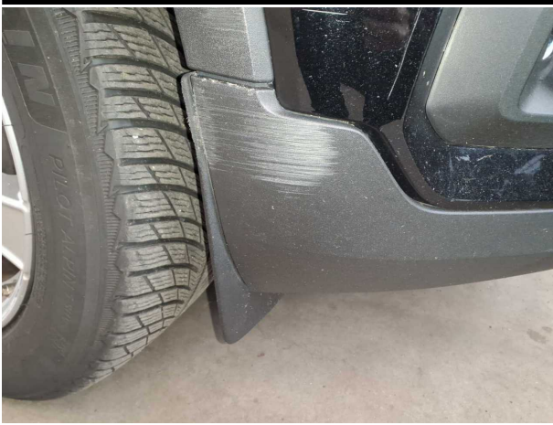
Damage #5: Front bumper: Spoiler - Abrasion - Replace
