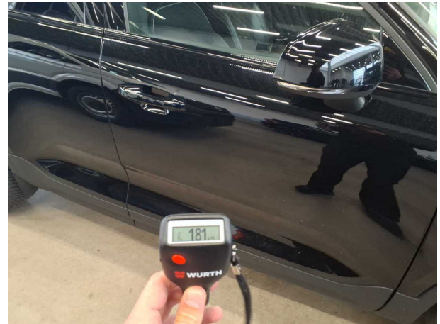
Repainting 4: Door - front right side
