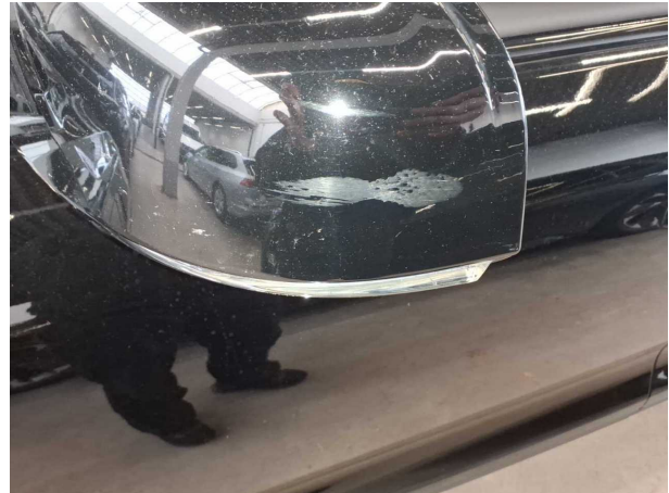
Damage #2: Wing mirror - left side: Mirror housing - Paint defect - Smart repair
