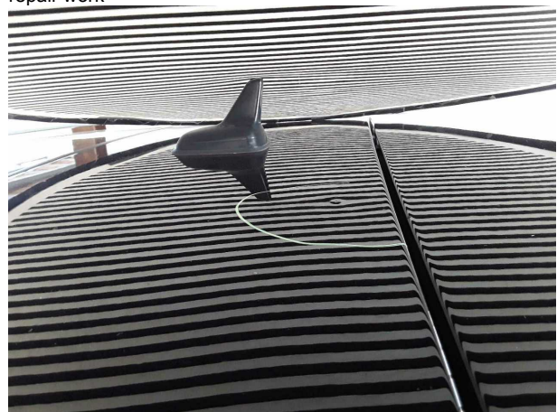
Damage #3: Roof: Roof - dent(s) - Smooth repair work
