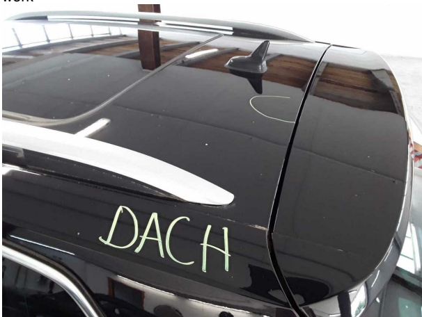
Damage #3: Roof: Roof - dent(s) - Smooth repair work
