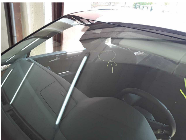
Damage #6: Vehicle glazing: Windscreen - Stone chips - Replace
