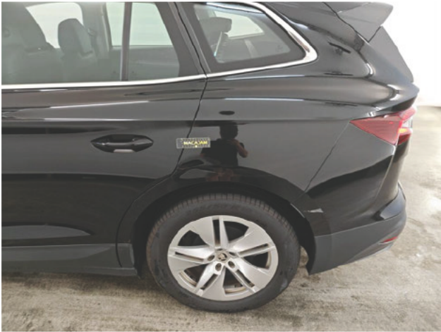
Wing RL Deformed / Strained Repair and paint (complete) Left
