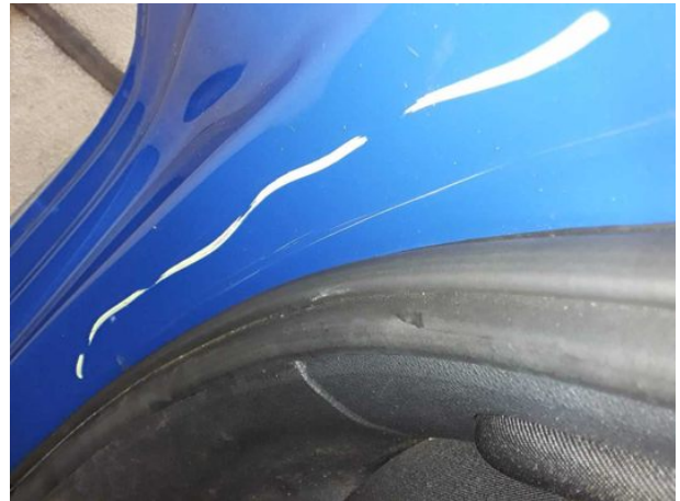
Damage #11: Side panel - rear right side: Sill - Dent / paintcoat damage - Repair and paint
