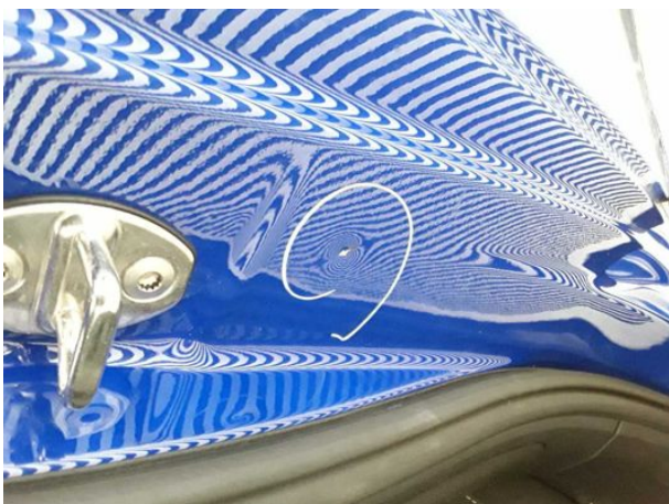
Damage #8: Side panel - rear left side: Sill - Dent / paintcoat damage - Smart repair
