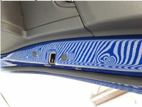
Damage #13: Door - rear right side: Door - Dent / paintcoat damage - Repair and paint
