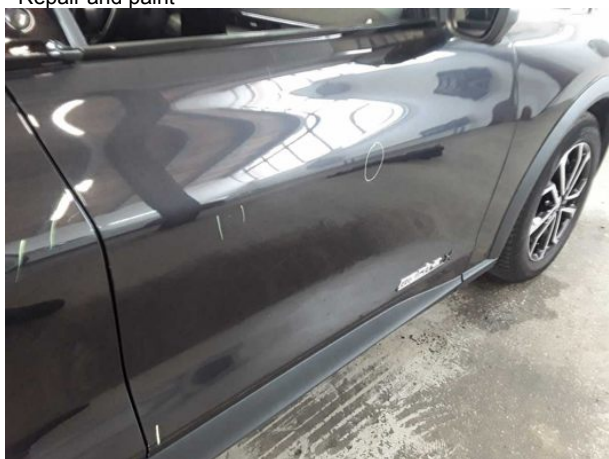
Damage #12: Door - front right side: Door - Dent / paintcoat damage - Repair and paint
