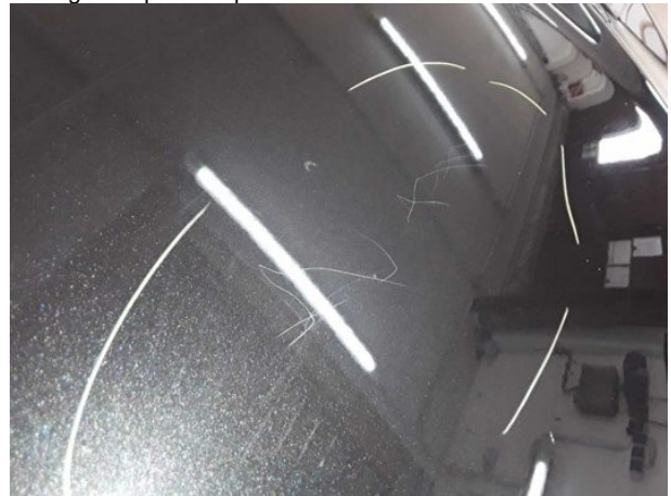
Damage #13: Bonnet: Bonnet - Scratched - Repair and paint
