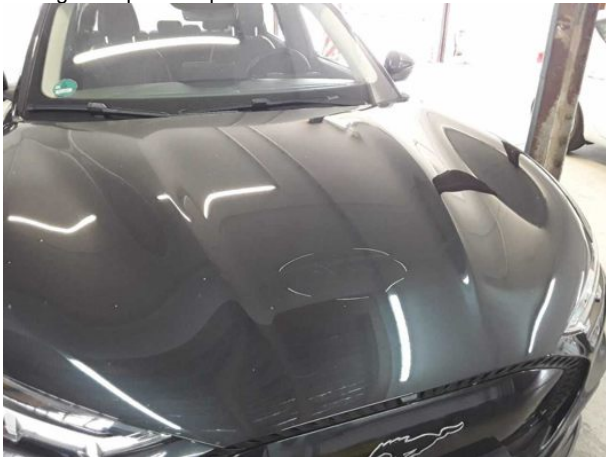
Damage #13: Bonnet: Bonnet - Scratched - Repair and paint
