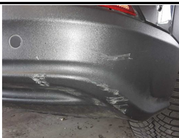
Damage #5: Rear bumper: Spoiler - Scratched - Replace
