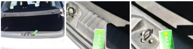
Rear roof pillar covering R, Broken, Replace
