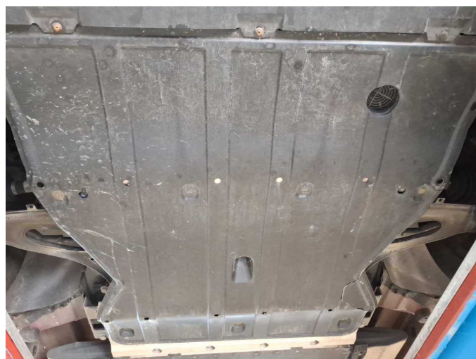
Damage 12: Engine: Engine cowling lower front - Broken / torn - Replace
