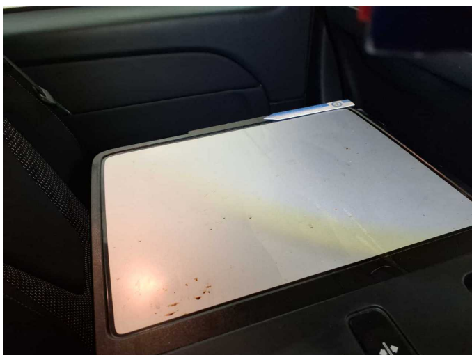
Damage 13: Equipment: tabletop (+ verschmutzt) - Scratched - Replace
