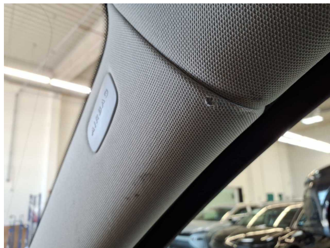
Damage 11: Trim / covers: A-pillar - interior trim - right side - Damaged - Replace
