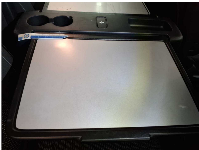
Damage 13: Equipment: tabletop (+ verschmutzt) - Scratched - Replace
