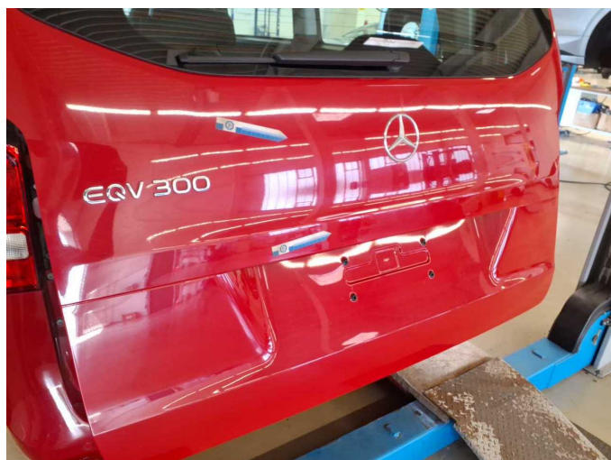
Wear and tear 3: Boot lid / rear door: Boot lid glazed - dent(s) - No deduction
