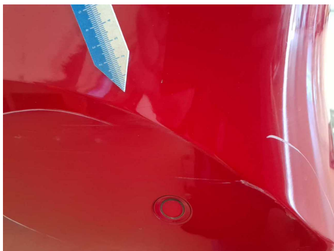
Damage 19: Rear bumper: Bumper with Parktronic - Scratched - Paint
