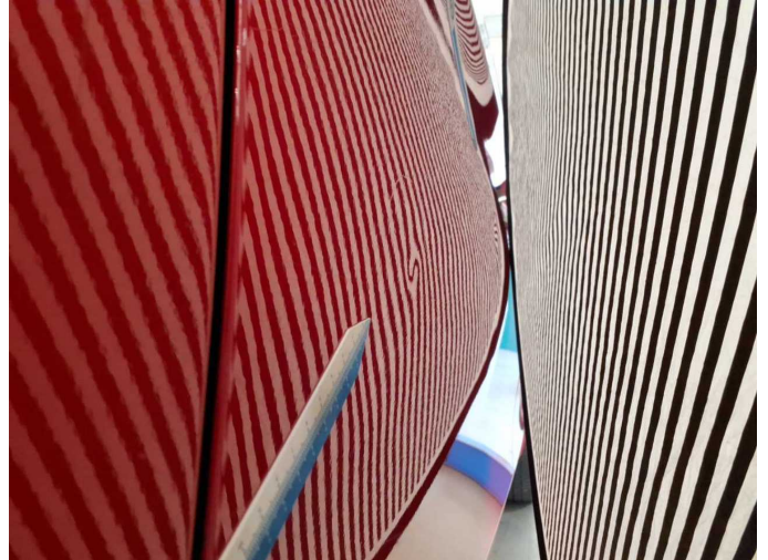
Damage 21: Sliding door, right: Sliding door with glass panel - dent(s) - Repair and paint
