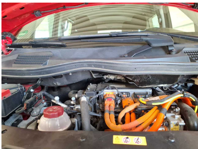
Damage 14: Cab: Insulation lining (+ Motorhaube) - Damage caused by marten / rodent - Replace
