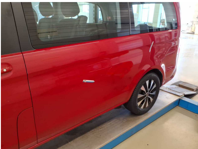
Damage 22: Side panel - rear left side: Side panel (wellig) - Unprofessionally repaired - Repair and paint
