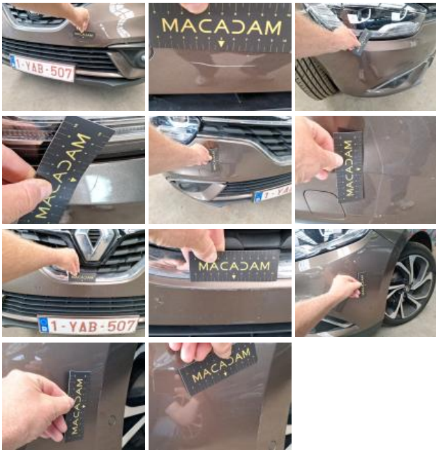
Bonnet, Dent(s) and scratch(es), Repair and paint (complete)
