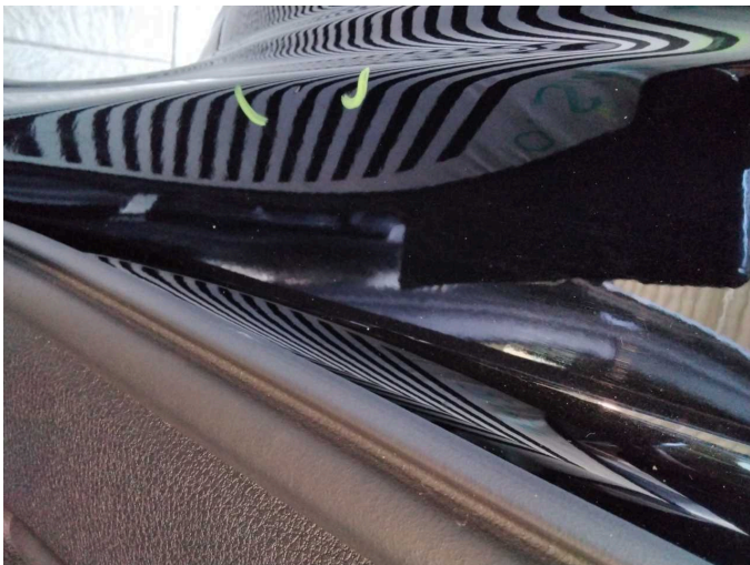
Damage 4: Body: C-pillar - right side - Dent / paintcoat damage - Smart repair
