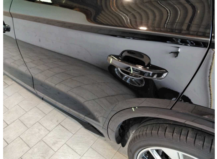
Damage 1: Door - rear left side: Door handle - outside - Scratch(es) - Smart repair
