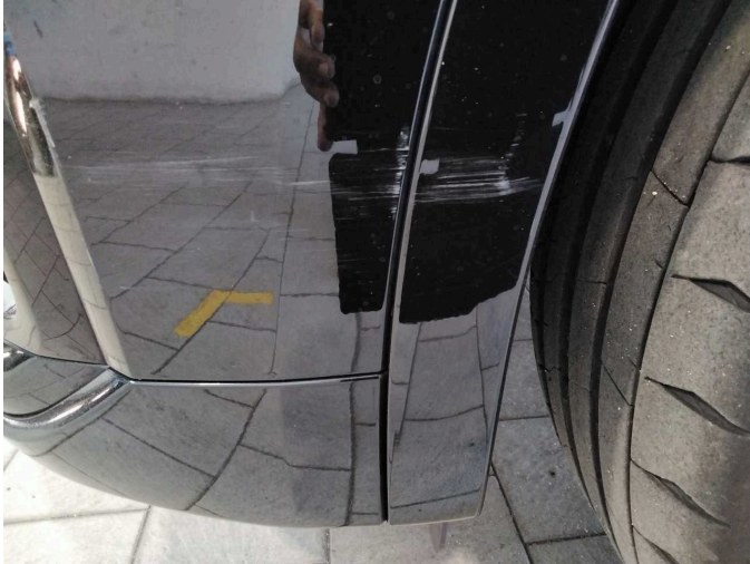
Damage 6: Mudguard - left side: Wheel well extension - Scratch(es) - Smart repair
