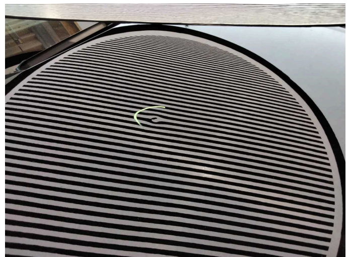
Damage 3: Bonnet: Bonnet - dent(s) - Smooth repair work
