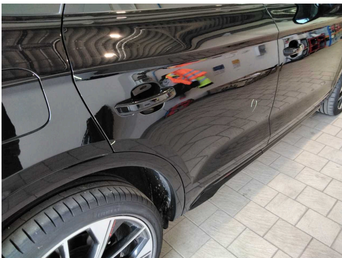
Wear and tear 3: Door - rear right side: Door - dent(s) - No deduction
