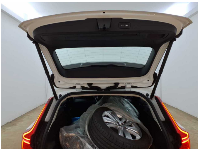
Damage 2: Boot lid / rear door: Gas pressure damper (Motoren, schwergängig, Knarren) - Functional / admissibility - Perform diagnosis
