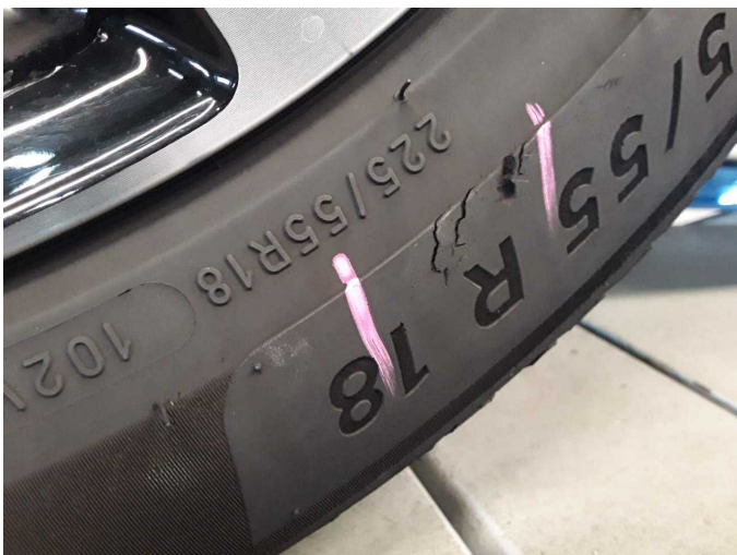
Damage 5: Wheel / tyres: Tyre - front left side (nicht fahrbereit) - Damaged - Replace
