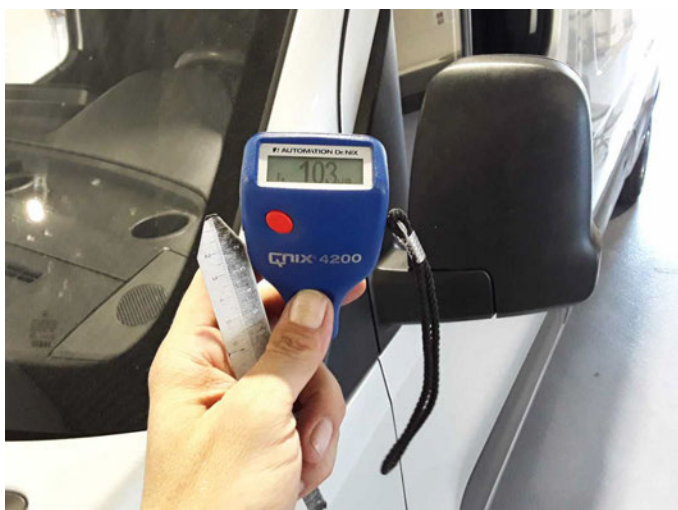
Dachholm links: 103 µm
