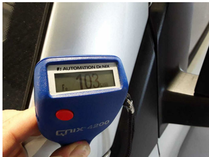
Dachholm links: 103 µm
