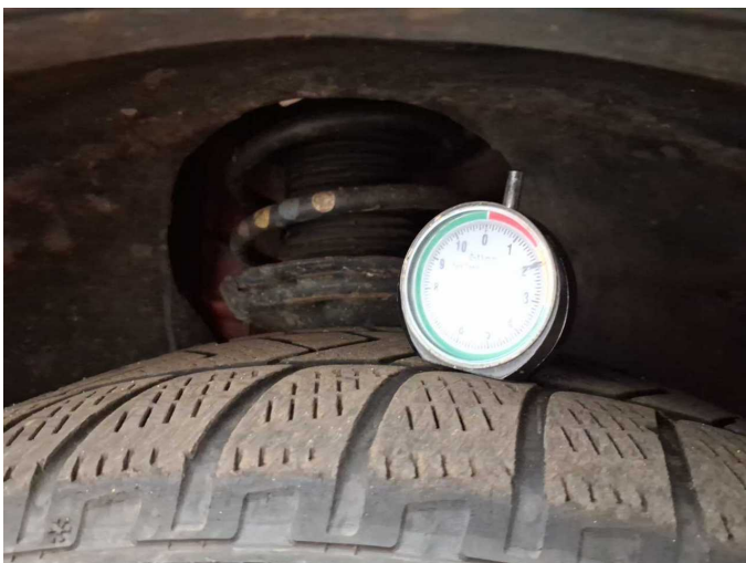
Damage 5: Wheel / tyres: Tyre - front right side - Does not meet the leasing specifications - Replace
