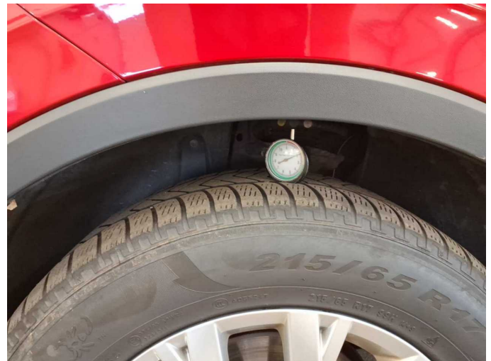
Damage 4: Wheel / tyres: Tyre - front left side - Does not meet the leasing specifications - Replace
