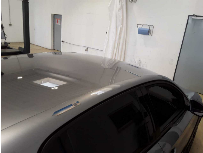
Damage 4: Roof: Roof - dent(s) - Smooth repair work
