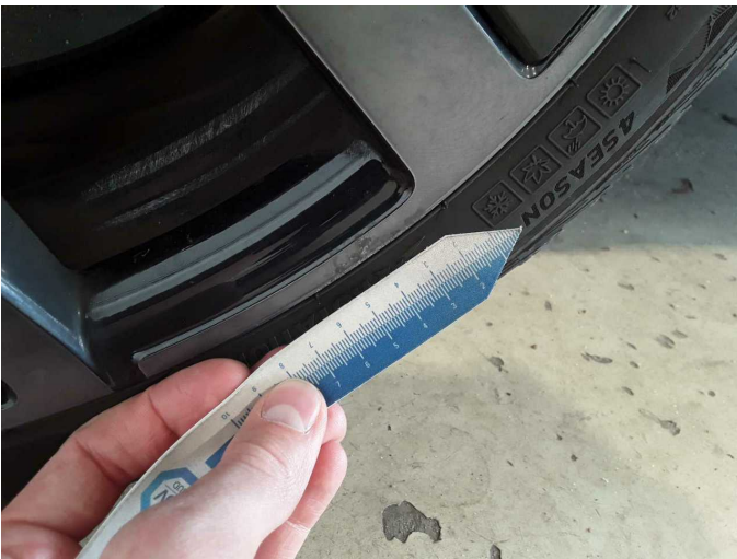
Damage 7: Wheel / tyres: Alloy rim - front left side - Scratch(es) - Replace
