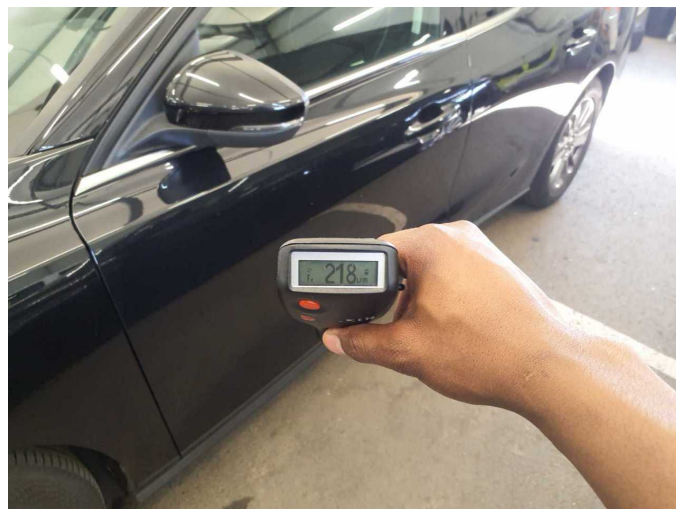
Repainting 1: Door - front left side
