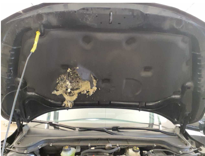
Damage 2: Bonnet: Insulation lining - Damage caused by marten / rodent - Replace
