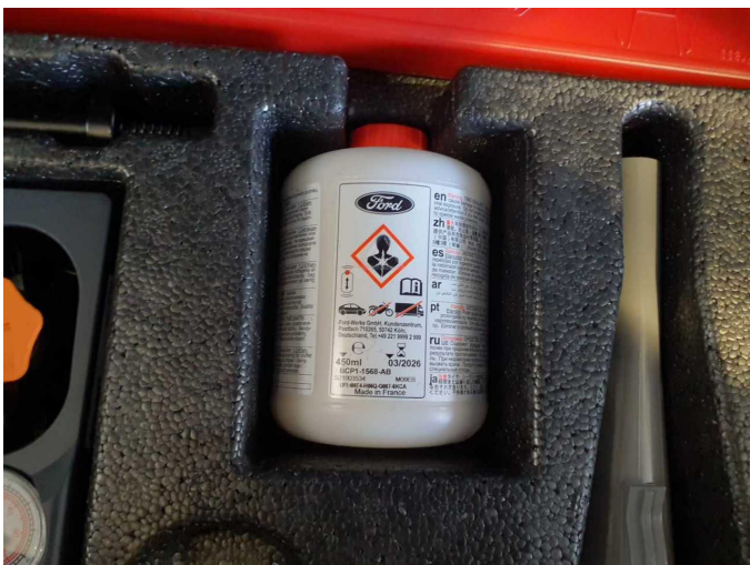
Damage 1: Equipment: Tirefit filler - Expired - Replace
