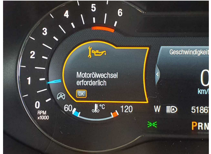
Damage 6: Misc.: Inspection / maintenance - Due - Replace
