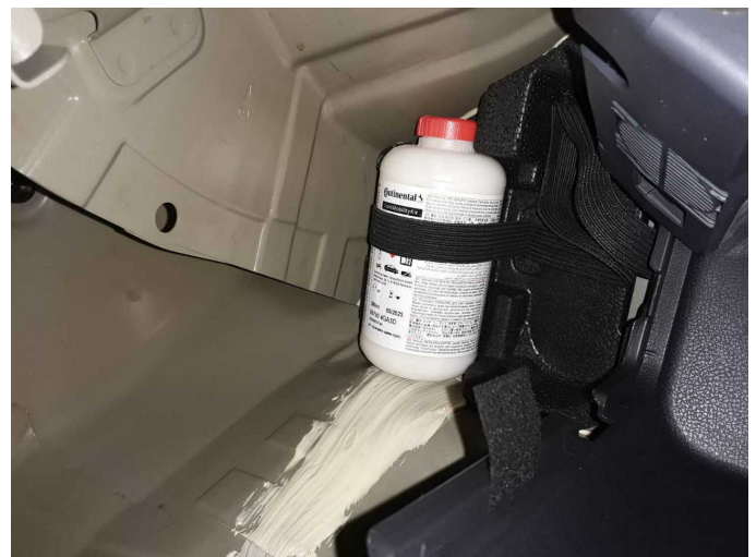
Damage 3: Equipment: Tirefit filler - Expired - Replace
