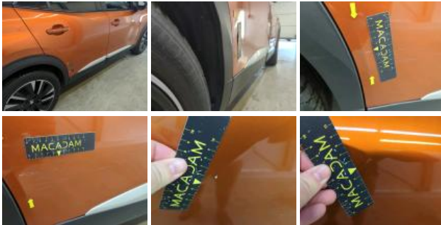
Wheel arch cover RR, Scratch(es), Replace
