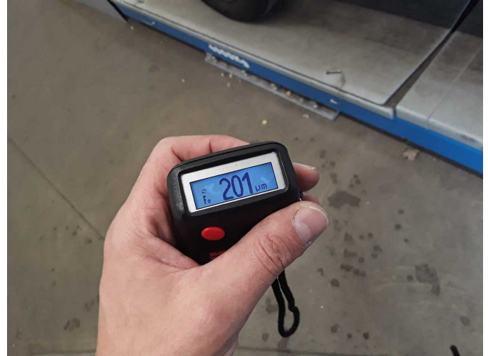
Repainting 1: Side panel - rear right side, Door - rear right side, Door - front left side
