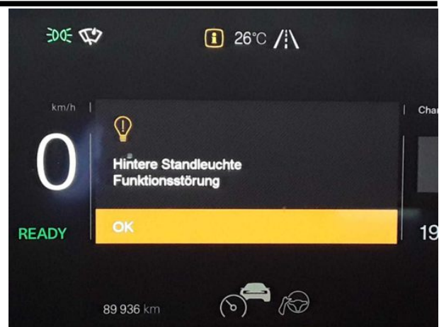
Damage #9: Electronic systems: Electronic systems (Beleuchtung) - Specify findings - Perform diagnosis
