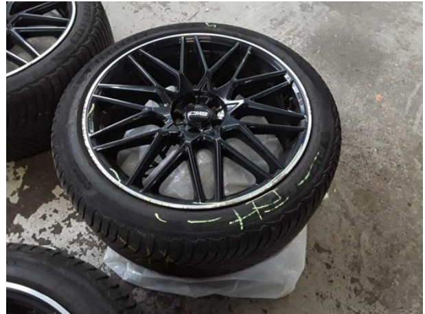
Damage #1: 2nd wheel set: 1 tyre - Abrasion
