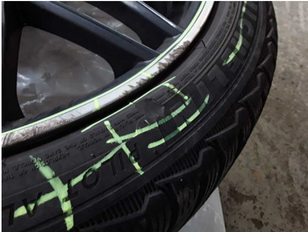
Damage #1: 2nd wheel set: 1 tyre - Abrasion
