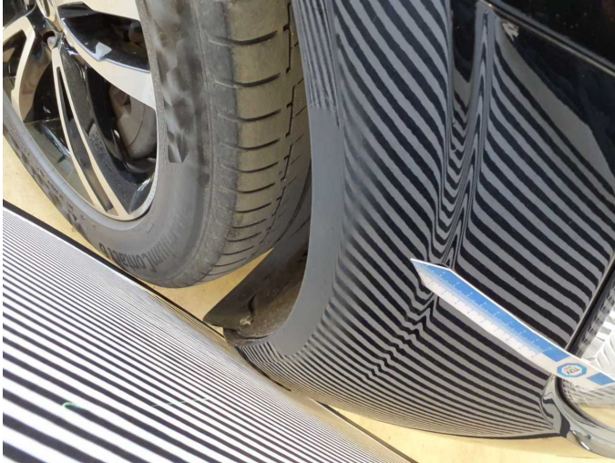
Damage 11: Front bumper: Front bumper (Matt und kantig) - Unprofessionally repaired - Repair and paint
