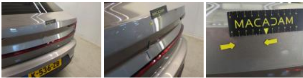
Tailgate / Boot, Dent(s), Repair and paint (complete)
