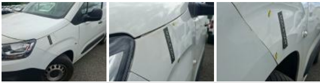
Door FL, Dent(s), Repair and paint (complete)
