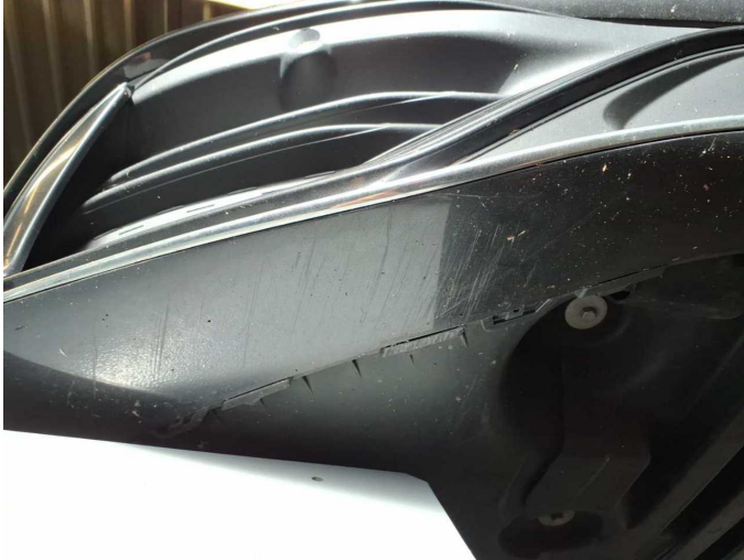
Damage 4: Front bumper: Front bumper - Scratched - Smart repair
