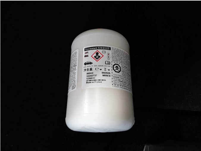
Damage 1: Equipment: Tirefit filler - Expired - Replace
