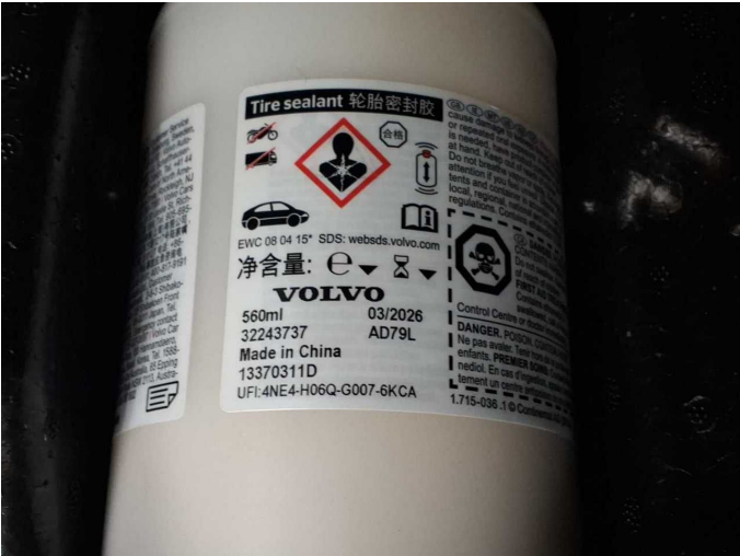
Damage 1: Equipment: Tirefit filler - Expired - Replace
