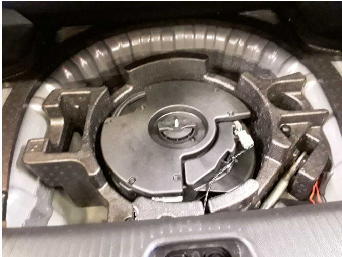
Missing part 1: Equipment: Tirefit complete - Missing - Replace
