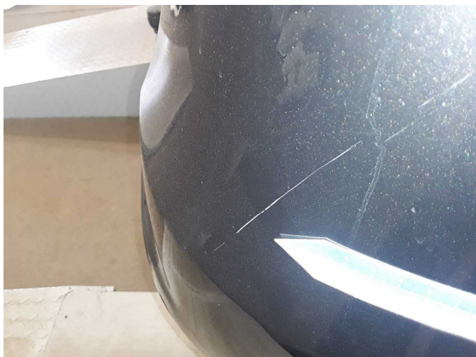
Damage 6: Rear bumper: Rear bumper - Scratch(es) - Paint
