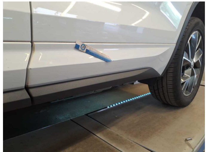
Wear and tear 1: Door - rear left side: Brightware - lower - Stone chips - No deduction
