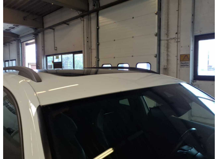
Damage 4: Roof: Roof - Stone chips - Paint
