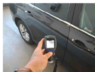
Paint thickness Door RR
