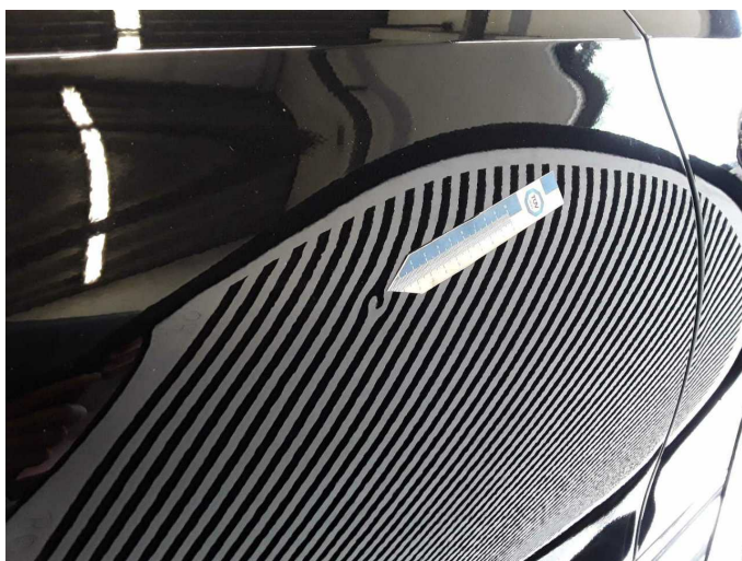
Wear and tear 7: Door - rear right side: Door - dent(s) - No deduction
