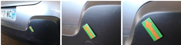
Bumper moulding R, Scratch(es), Replace
