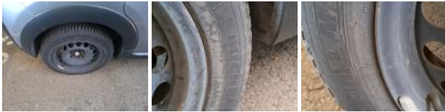
Wheel cover RR, Missing, Replace
