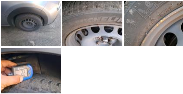
Wheel cover FR, Missing, Replace
