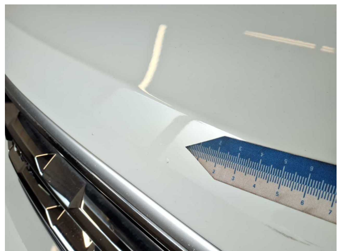
Damage 5: Bonnet: Bonnet - Corrosion - Repair and paint
