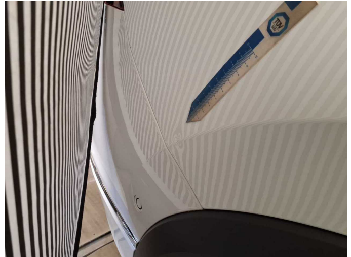
Damage 4: Side panel - rear right side: Side panel - Dent / paintcoat damage - Repair and paint
