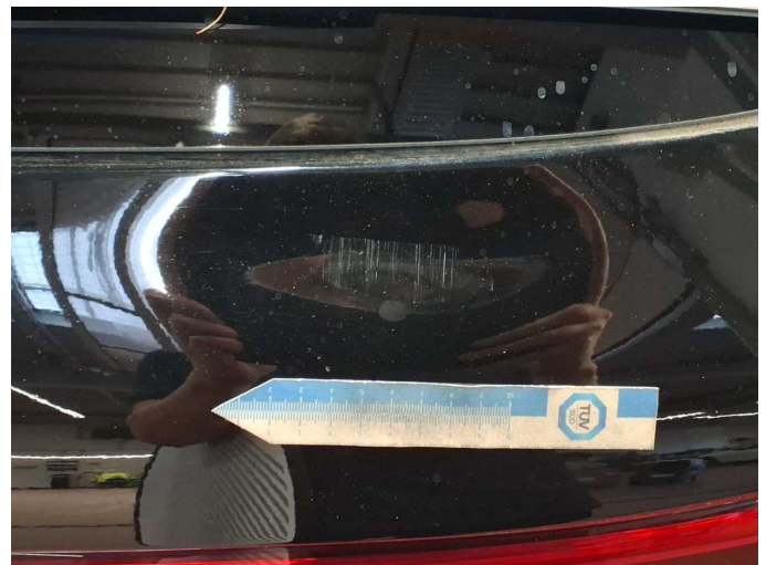
Damage 11: Boot lid / rear door: Boot lid (Knick) - Deformed - Repair and paint
