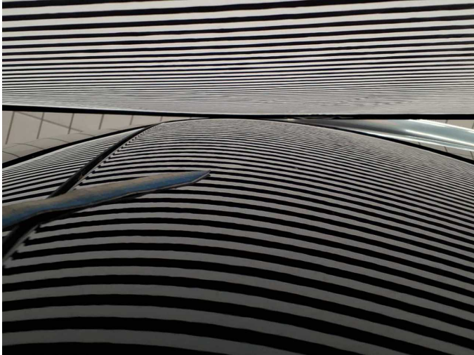
Damage 3: Roof: Roof - dent(s) - Smooth repair work
