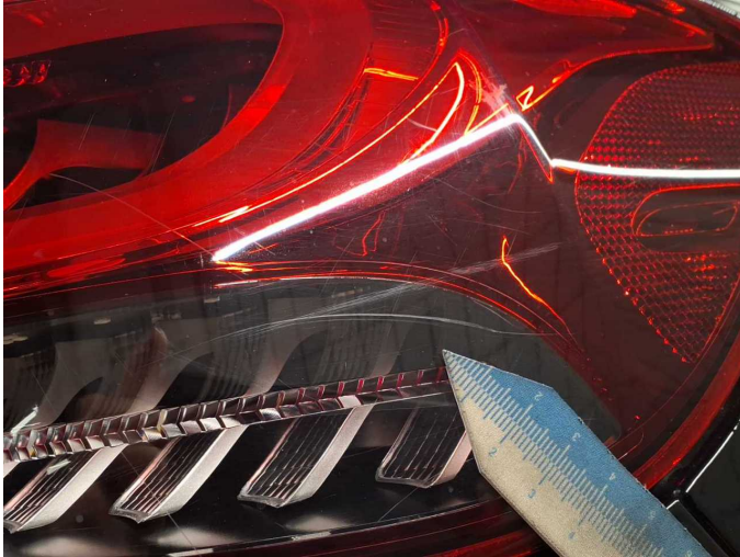
Damage 8: Tail light: Tail lamp - right side (Optischer Mangel) - Scratch(es) - Replace
