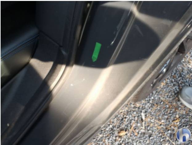
4. Tür Hinten - Links Kratzer - Smart Repair
