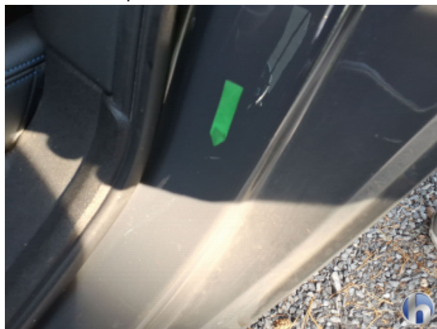
4. Tür Hinten - Links Kratzer - Smart Repair
